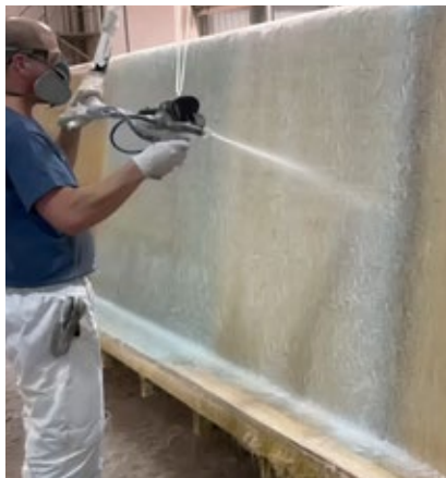
5 Simultaneous Resin & Fiber Spray
